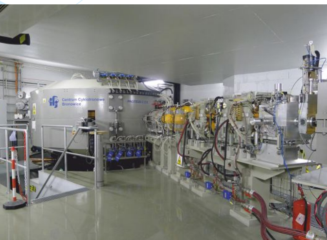
The Proteus C-235 Cyclotron which accelerates protons to energies of up to 230 MeV, with its beam delivery systems for medical and scientific research applications
